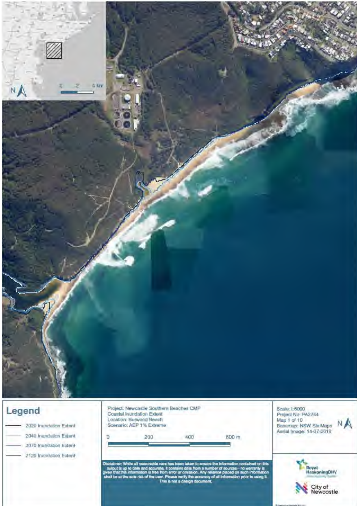
Figure 33: 1% AEP extreme Inundation Hazard extent map Burwood Beach
