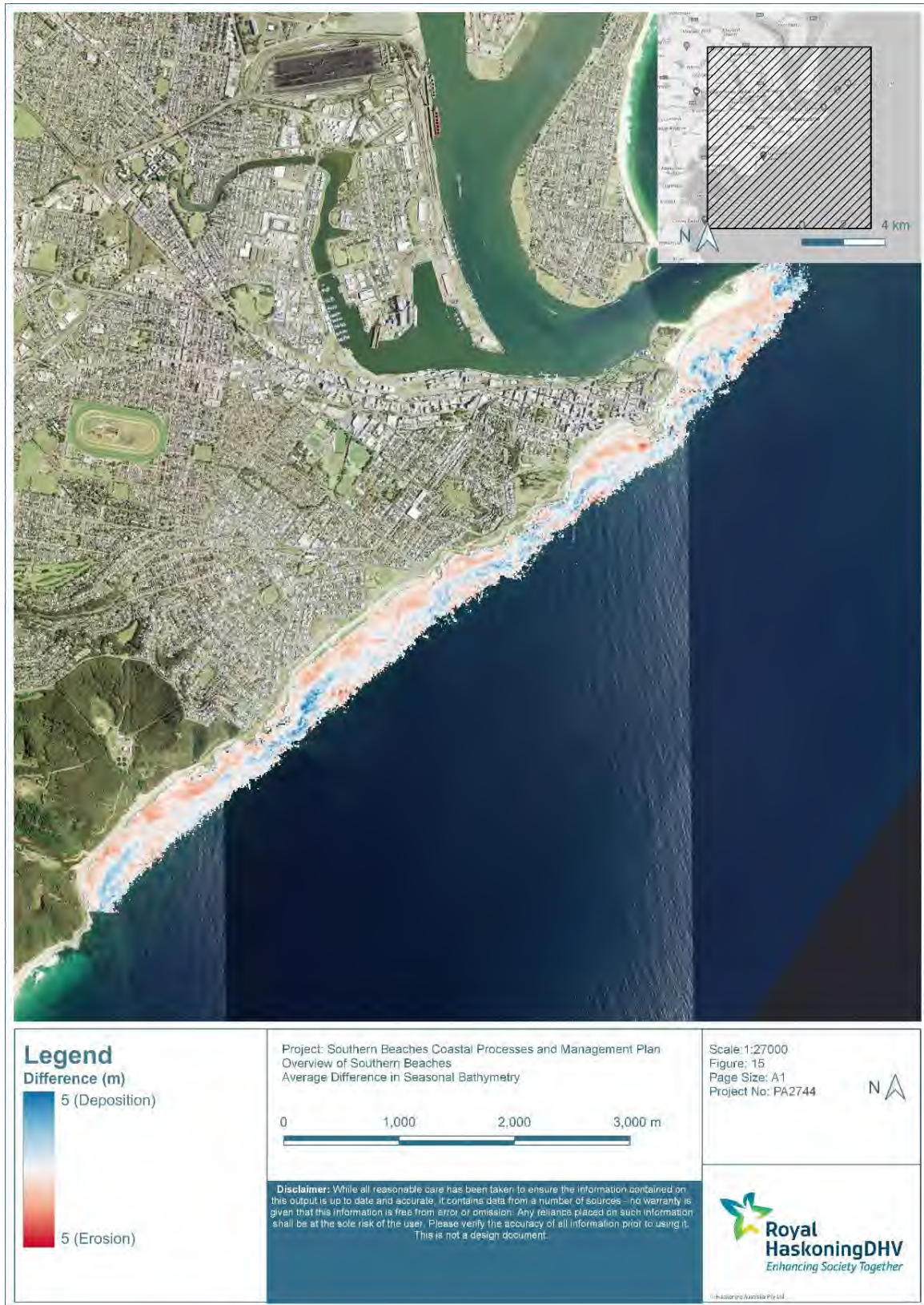
Figure 24: A plot showing the elevation difference of the average summer bathymetry subtracted from the average winter bathymetry. Blue values represent areas where the winter bathymetry is higher than the summer bathymetry.
