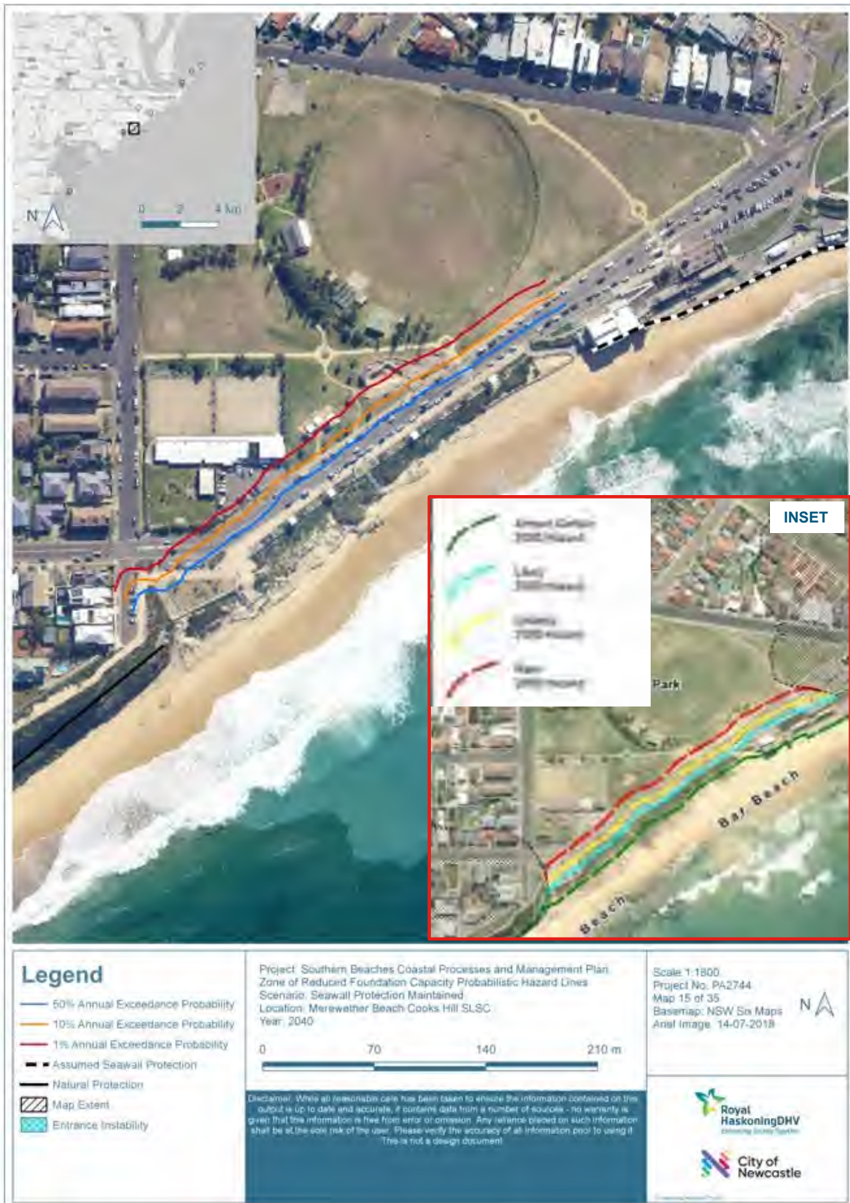
Figure 68: 2040 coastal erosion hazard lines for Bar Beach area and BMT WBM (2014) 2050 hazard lines (INSET)
