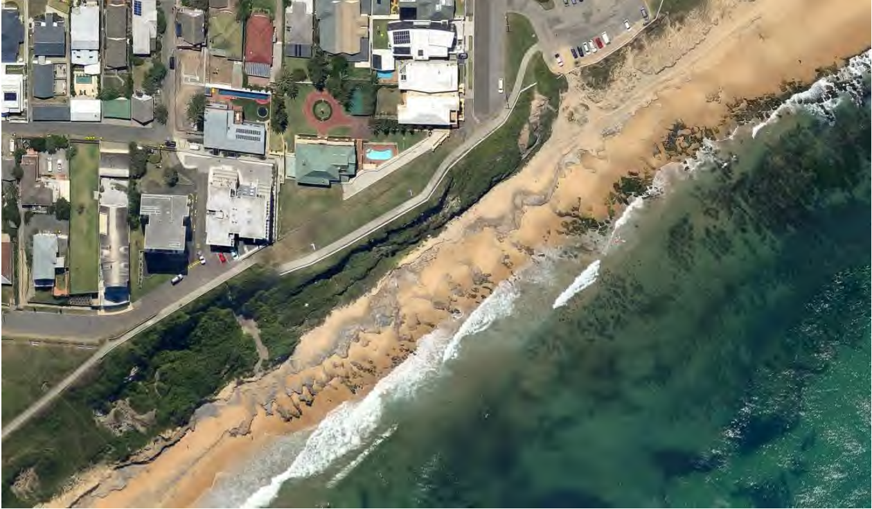
Figure 9: Near Map image, March 2013, showing significant rock underlying beach at The Cliff at the southern end of Bar Beach.
