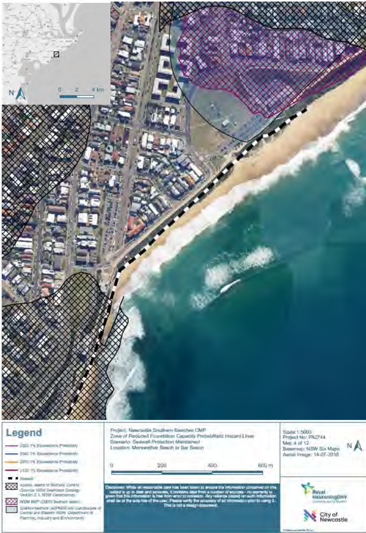
Figure 59: Summary 1% AEP Coastal erosion hazard lines for Merewether to Dixon Park Beach (seawalls maintained scenario).
