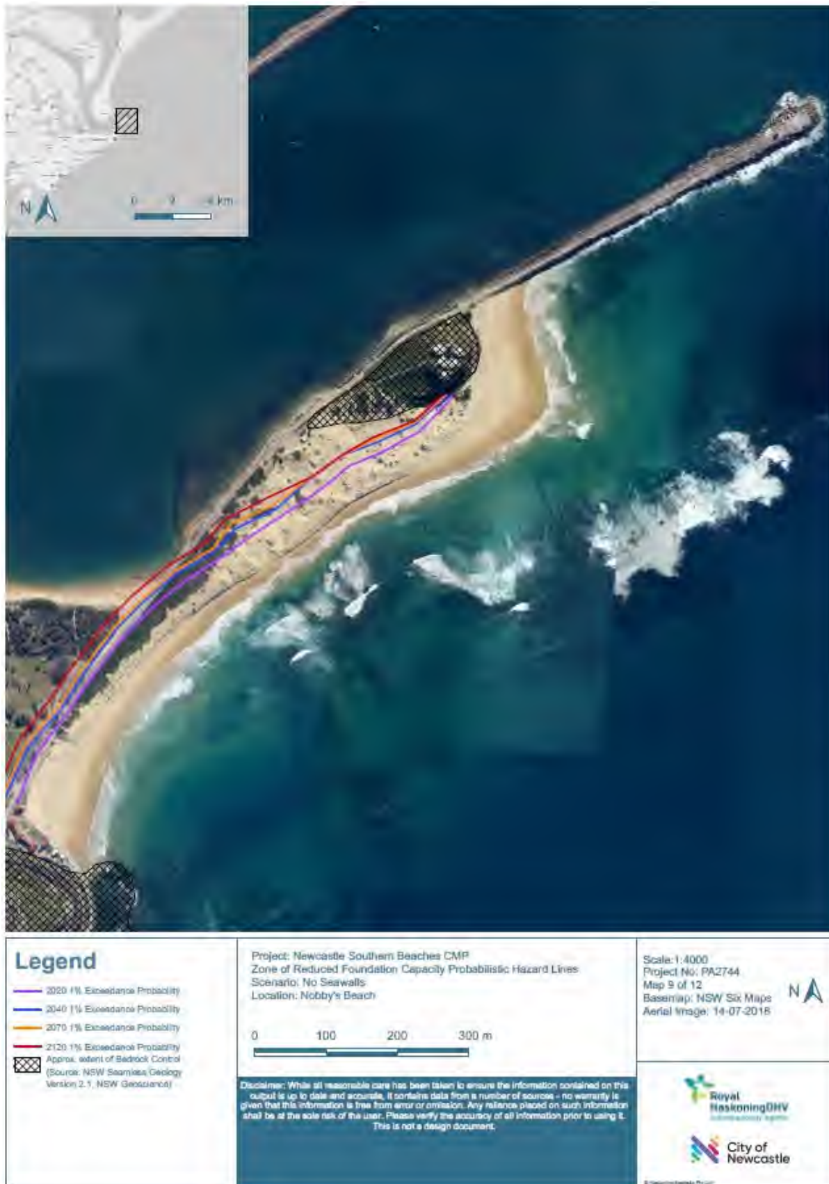
Figure 64: Summary 1% AEP Coastal erosion hazard lines for Nobbys Beach (no seawalls scenario).
