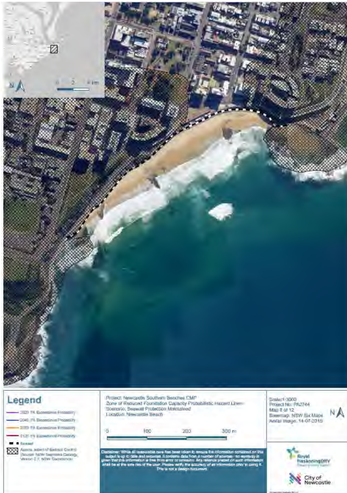
Figure 63: Summary 1% AEP Coastal erosion hazard lines for Newcastle Beach (seawalls maintained scenario).
