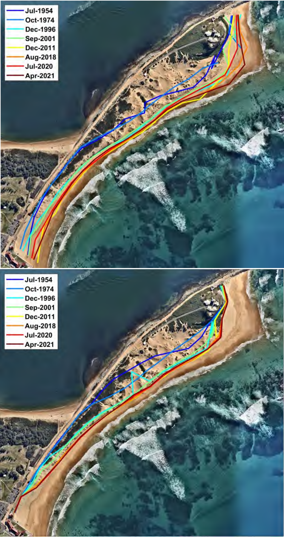
Figure 20: Position of 2m and 4m AHD contours (top and bottom photos respectively) for Nobbys Beach
