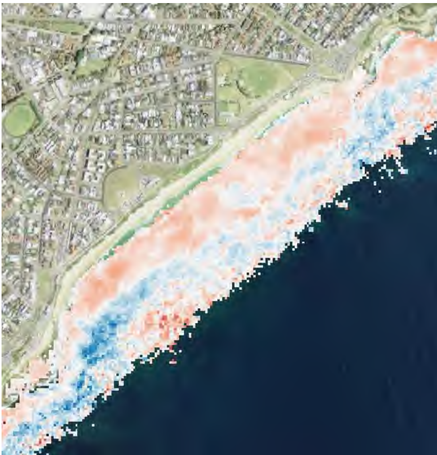
Figure 27: Detailed view of Mereweather Beach and Bar Beach showing the elevation difference of the average summer bathymetry subtracted from the average winter bathymetry. Blue values represent areas where the winter bathymetry is higher than the summer bathymetry.
