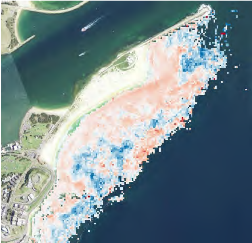
Figure 28: Detailed view of Nobbys Beach showing the elevation difference of the average summer bathymetry subtracted from the average winter bathymetry. Blue values represent areas where the winter bathymetry is higher than the summer bathymetry.
