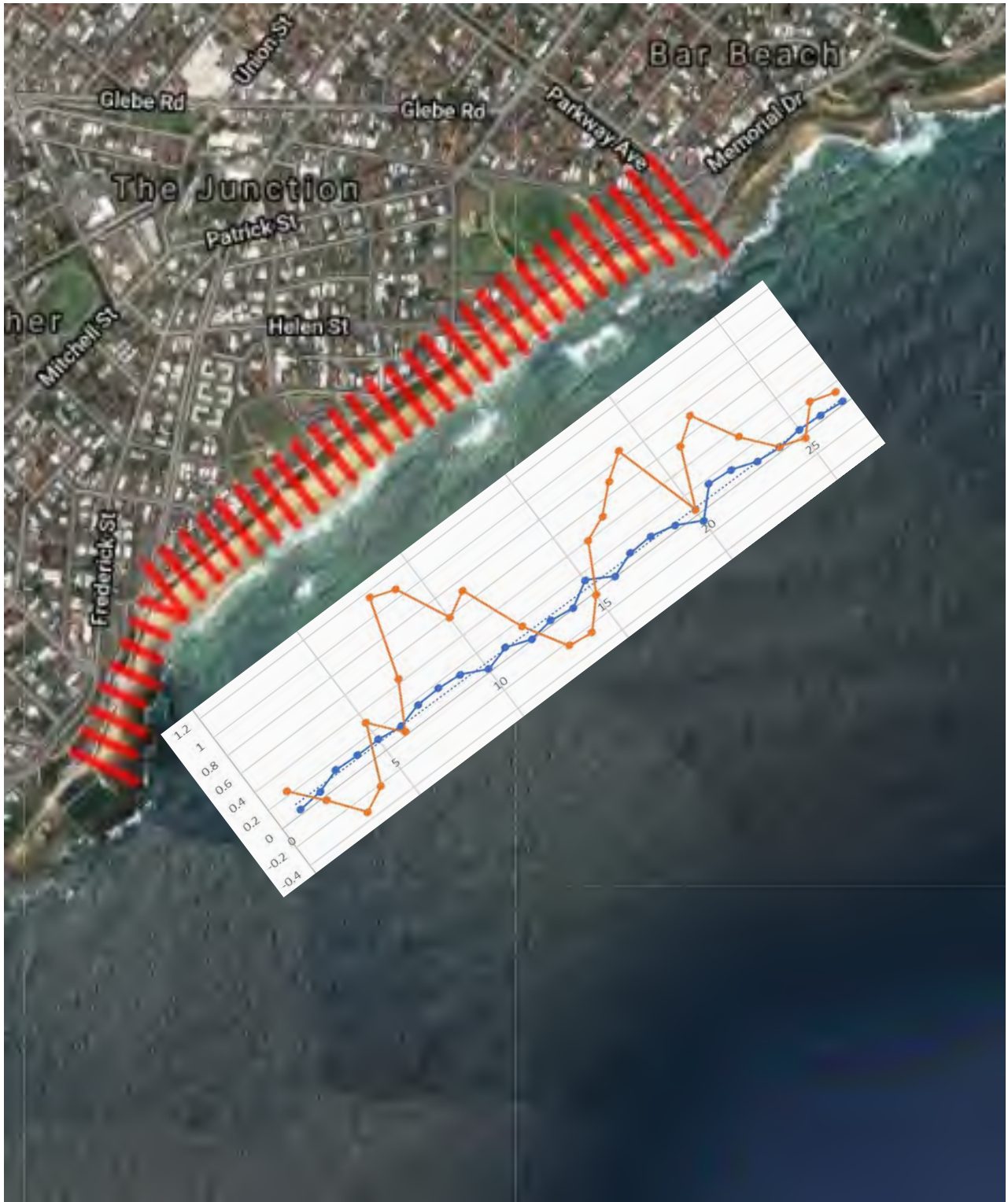
Figure A3: Block 3 John Parade, Dixon Park and Bar Beach volume change, above 0m AHD in m 3 /m/year (orange line) and 4m AHD contour movement in m/year (blue line) for 1954-2021 (positive values indicating accretion/ progradation and negative values indicating erosion/recession).
