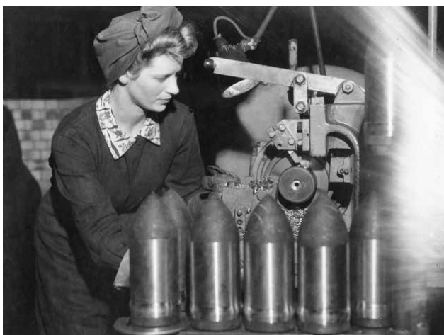
'Before the war, this girl [sic] was a shop assistant. Now, after a short period of training, she is operating a lathe in a munitions factory. This picture shows her at work, turning the copper driving band on 20-pounder anti-tank shots. She has been identified as Elsie Myra (Judy) Richards of Newcastle, NSW.' Photograph by Clifford Bottomley, 4 September 1942. (Source: Australian War Memorial, 03178)
