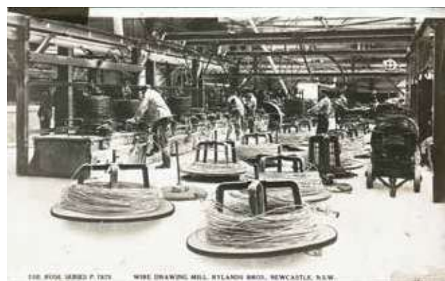
Rose Series postcard of wire drawing mill, Rylands Bros, Newcastle, 1910s. (Source: UON, Living Histories, A5194-025.5)
