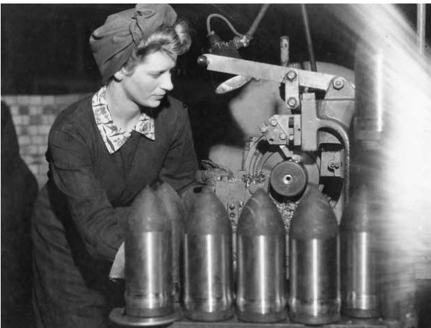
'Before the war, this girl [sic] was a shop assistant. Now, after a short period of training, she is operating a lathe in a munitions factory. This picture shows her at work, turning the copper driving band on 20-pounder anti-tank shots. She has been identified as Elsie Myra (Judy) Richards of Newcastle, NSW.' Photograph by Clifford Bottomley, 4 September 1942. (Source: Australian War Memorial, 03178)
